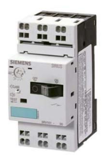
CIRCUIT-BREAKER SIZE S00, FOR MOTOR PROTECTION, CLASS 10, A-REL. 2.8...4A, N-REL. 52A, CAGE CLAMP CONNECTION, STANDARD SWITCHING CAPACITY
