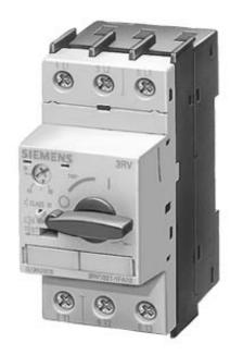
CIRCUIT-BREAKER SIZE S0, FOR MOTOR PROTECTION, CLASS 10, A-REL. 2.2...3.2A, N-REL.42A, SCREW TERMINAL, STANDARD SWITCHING CAPACITY
