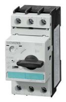
Circuit breaker size S0 for motor protection CLASS 10 A-release 3.5...5 A Short-circuit release 65 A Screw terminal Standard switching capacity !!! Phased-out product !!! Successor is SIRIUS 3RV2 Preferred successor type is >>3RV2011-1FA10<<
